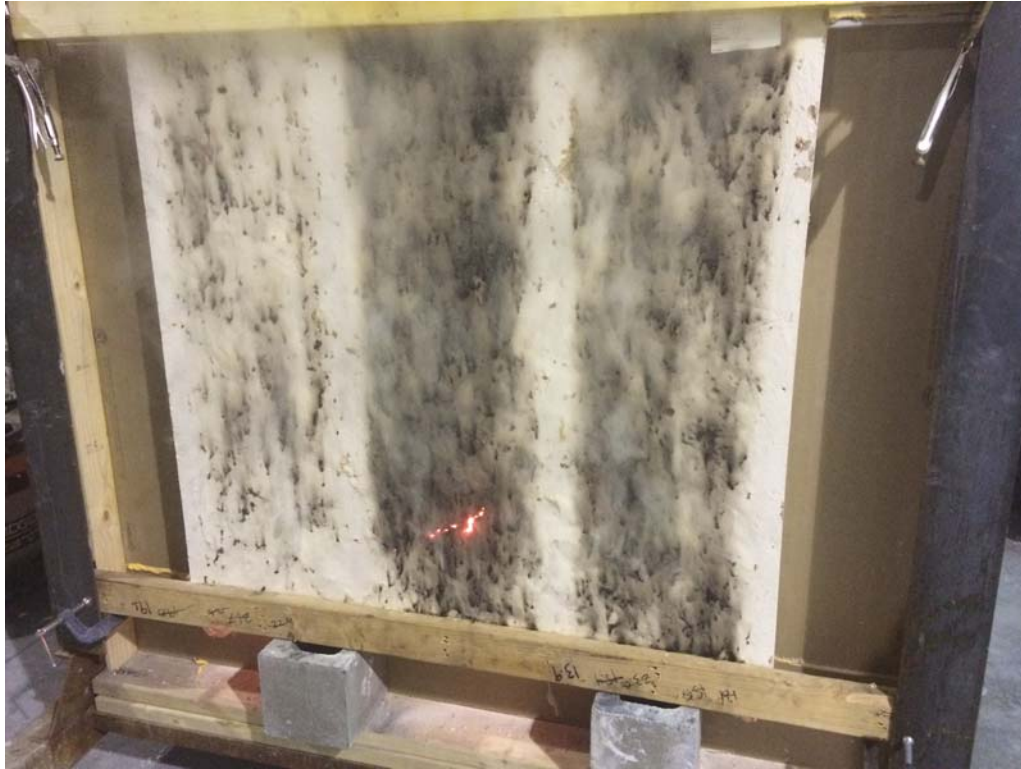
Figure 6: Unexposed Side at Termination of Fire Exposure
