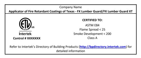
Figure 2 – Example of Factory Applicator Label
