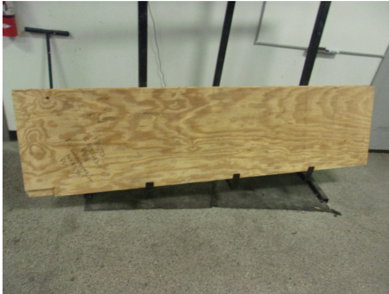
Photo No. 2 Exposed Surface of the Test Specimen (Pre-test)
