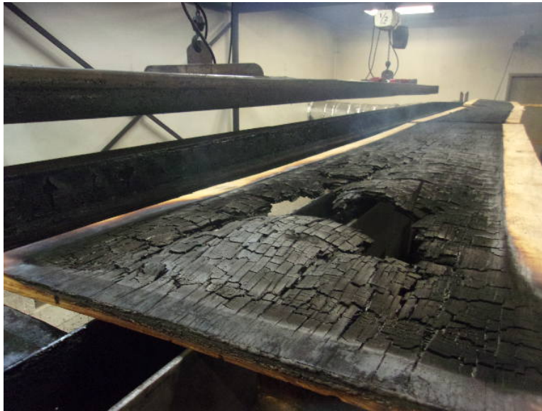
Photo No. 5 Exposed Surface of the Test Specimen (Post-test)
